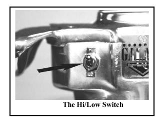
Use the high-speed setting for faster wood removal. Use the low-speed setting for finish cuts and custom work.
